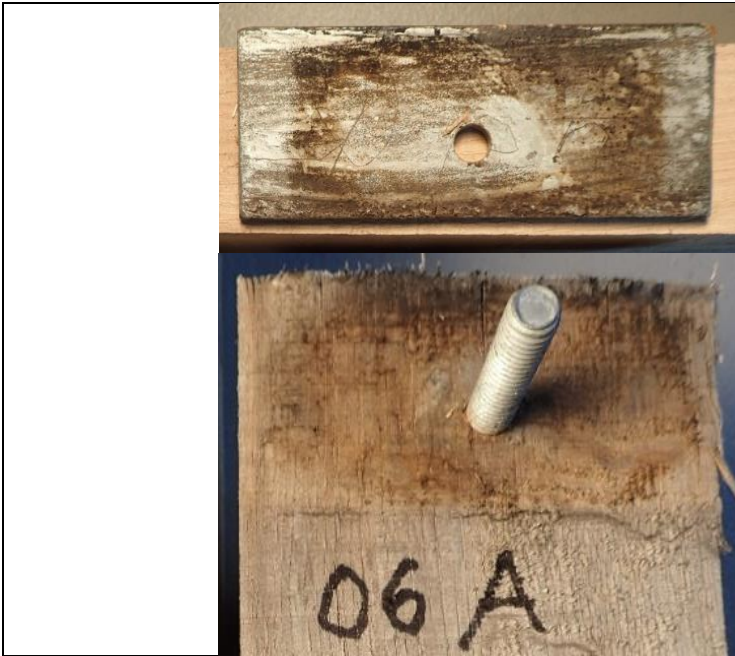
The upper portion of this image shows steel sample # 06 A with rust on the leg of the angle iron. The lower portion shows the piece of rough sawn white oak lumber that was attached to this piece of steel. It shows a transfer of rust from the steel angle iron.
