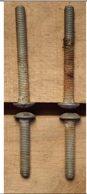
Sample of bolts that connected wood to steel for 1 year. Bolt through ACQ # (Top Left), Bolt through white oak (Top Right), EL2 (Bottom Left), and Bolt through MCA (Bottom Right)
